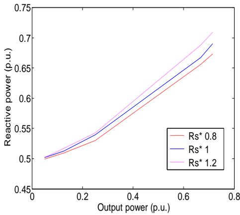
**Fig. 7** Variations of Reactive power with output power for different values of stator resistance.
