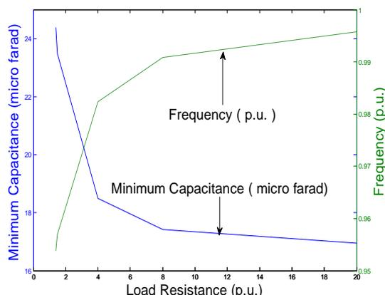
Fig. 6 Variations of minimum capacitance and frequency with load resistance.
