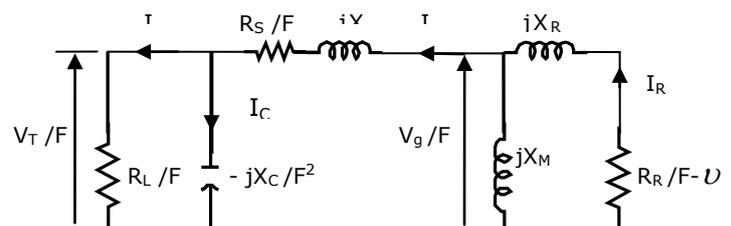
Fig. 1 Per-phase equivalent circuit of SEIG
