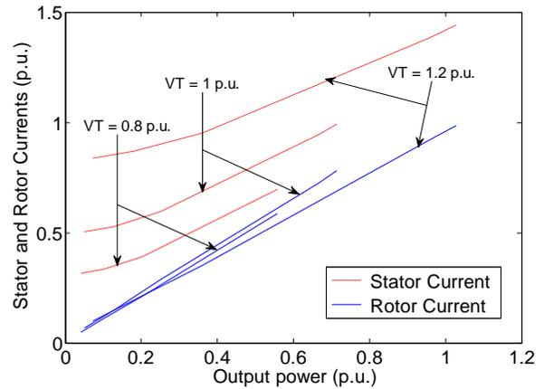
**Fig. 11** Variations of stator and rotor currents with output power for various constant terminal voltages and rated speed.
