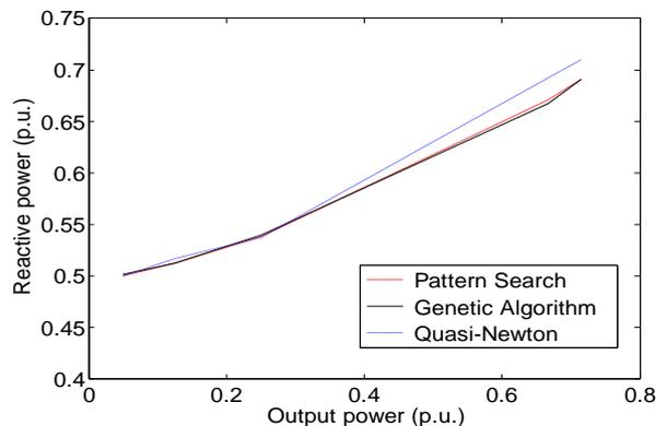
**Fig. 12** Variation of reactive power with output power.
