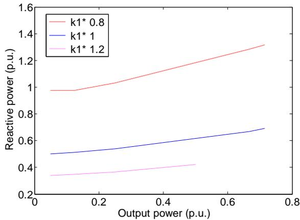
**Fig. 9** Variations of Reactive power with output power for different values of  $K_1$ .
