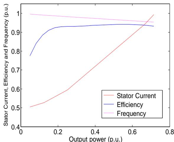
Fig. 5 Variations of stator current, efficiency and frequency with output power.
