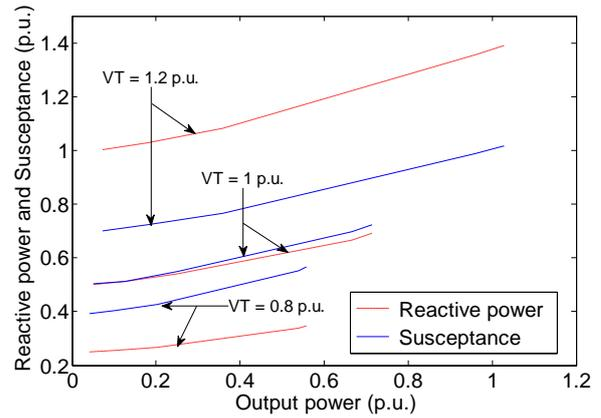
**Fig. 10** Variations of reactive power and capacitance in terms of susceptance with output power
