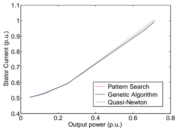
Fig. 14 Variations of stator current with output power.
