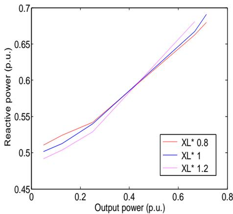
**Fig. 8** Variation of Reactive power with output power for different values of leakage reactance.
