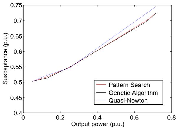
Fig. 13 Variations of susceptance with output power
