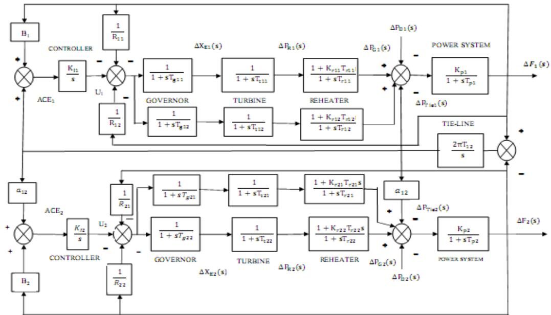
Fig. 2 Transfer function model of a TATURIPS
