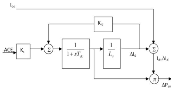
Fig. 4 Block diagram of SMES unit
