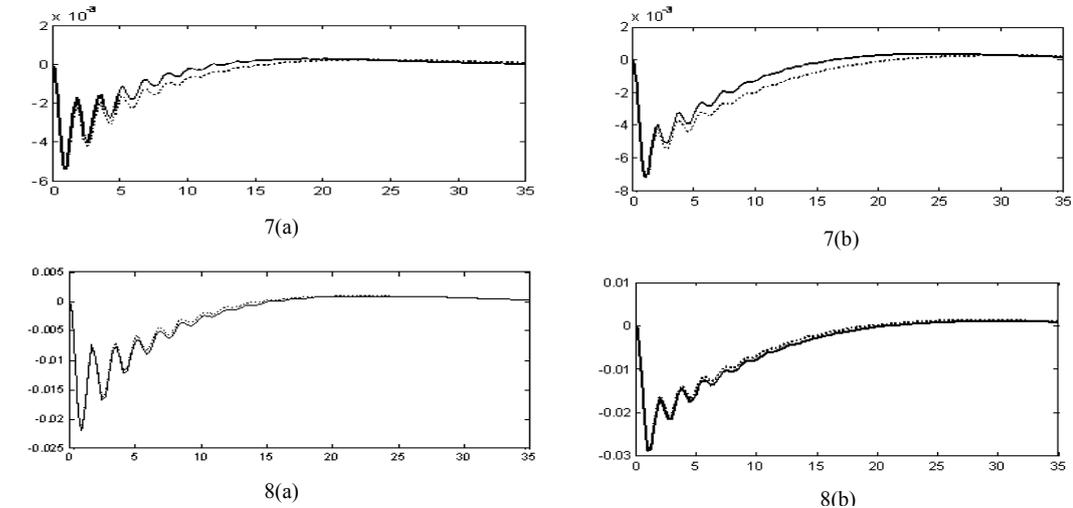
Fig. 8: 7(a),7(b) --- Tie-line Power deviations without and with SMES,both units in operation and Single unit in operation for a step load change of 1% 8(a),8(b) --- Tie-line deviations without and with SMES both units in operation and Single unit in operation for a step load change of 4%, Solid line (TATURIPS), Dotted line ( TATURIPS with SMES unit)
