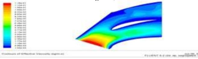
Figure 57: Contour of Effective Viscosity ( $\alpha = +6$  degrees)
