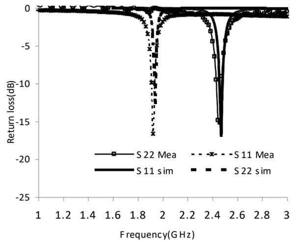
Fig.3: Simulated and measured S-parameter plot for the antenna
