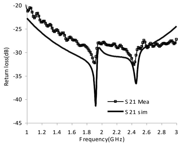
Fig. 4: simulated and measured S-parameter plot for isolation between ports
