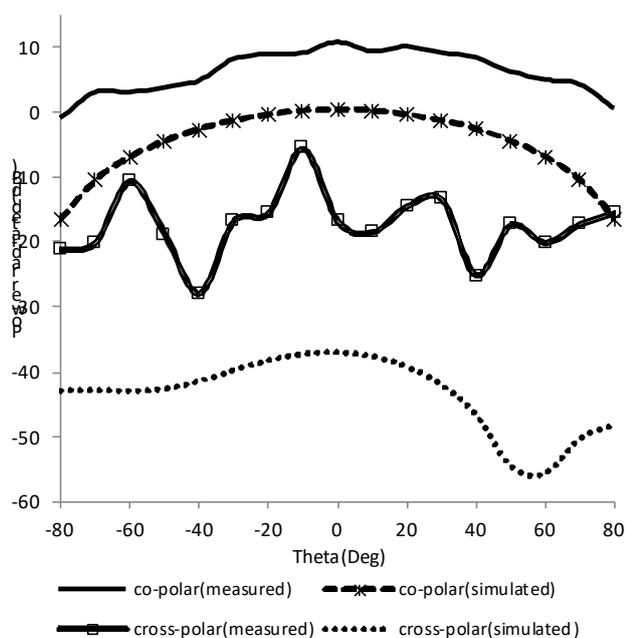
Fig.13: E-plane radiation pattern at 2.45GHz (with DMS)
