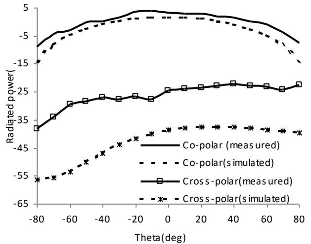
**Fig 12: E-plane radiation pattern at 1.95GHz (with DMS)**
