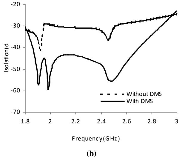
**Fig 11: comparison of Isolation between conventional and DMS integrated antenna (a) Simulated, (b) Measured**
