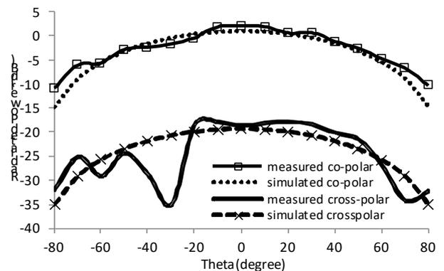
Fig.: 5 E-plane radiation pattern at 1.95 GHz
