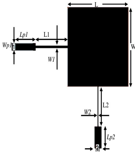
Fig.1: Schematic of rectangular patch antenna
