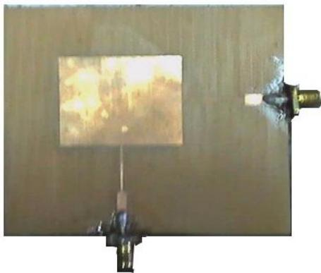
Fig.2: Photograph of rectangular patch antenna
