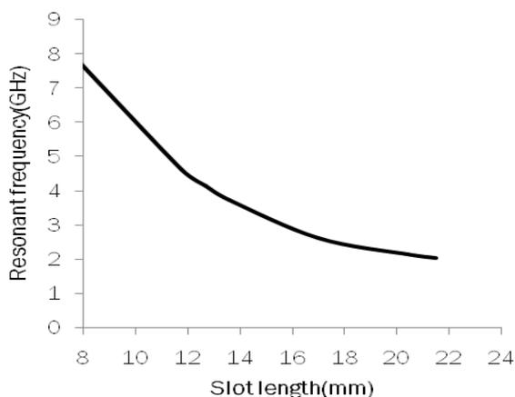
Fig.8: slot length vs Frequency graph for DMS
