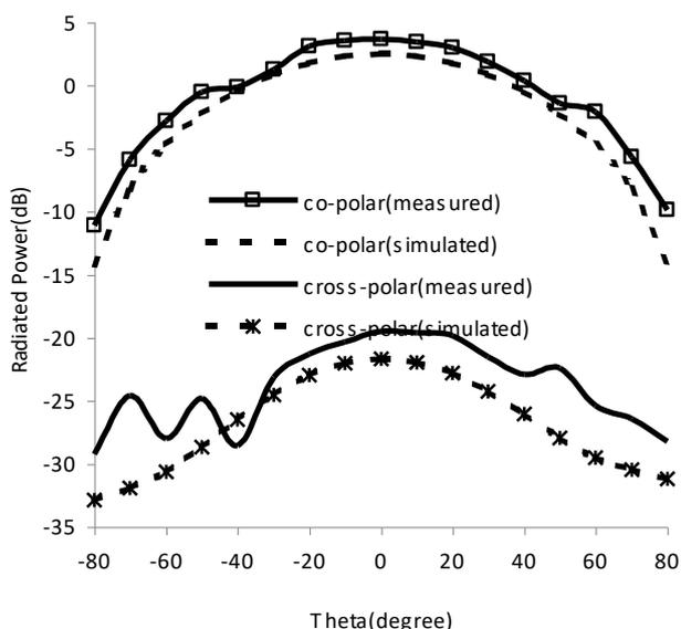
Fig.: 6 E-plane radiation pattern at 2.45 GHz
