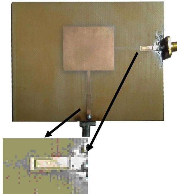
Fig.9: photograph of the fabricated antenna with DMS at both feed line
