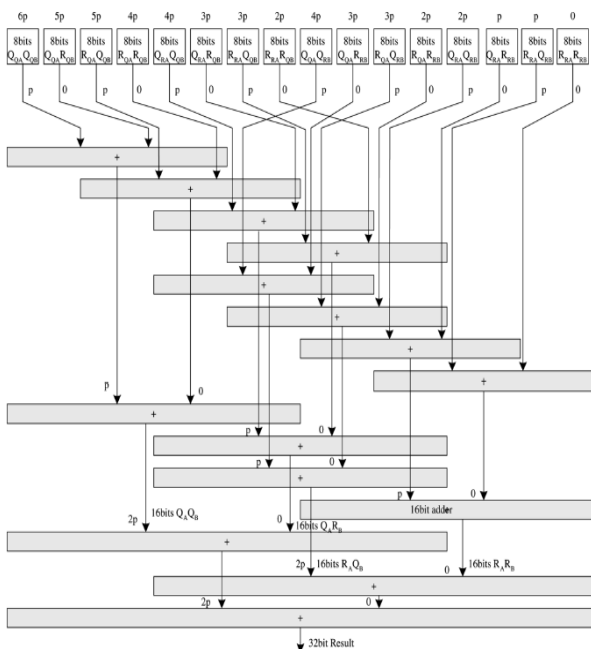
Fig. 2. Illustration of 2-input adder tree structure in the balanced composition process with W = 16 and p = 4.
