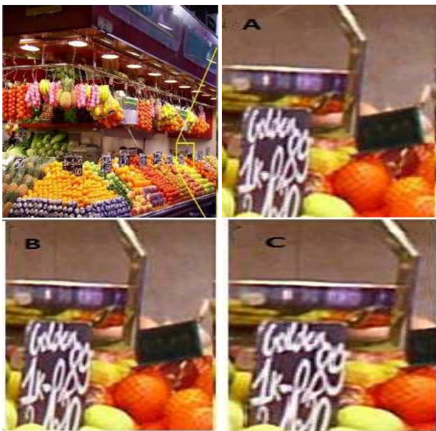
Fig 4. 4× upscaling of a 4 Megapixel image (not downsampled). A: Nearest neighbor enlargement showing a small detail at the original resolution. B: Same detail enlarged with ICBI: pixelization is removed without creating evident jaggies or artifacts, but the image appears oversmoothed. C: The same upscaled detail in B after a simple post-processing (selective smoothing and sharpening) enhancing the perceived quality of the printed image.
