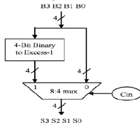
Fig. 3. 4-b BEC with 8:4 mux.
