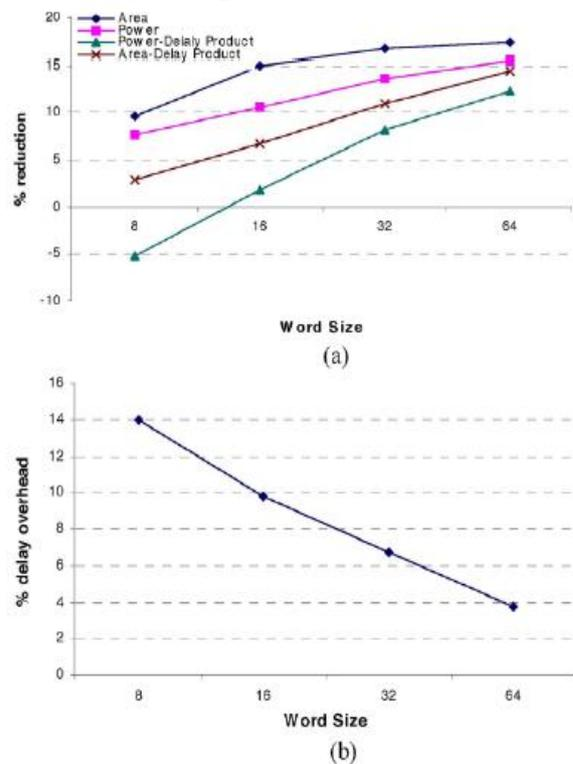
Fig. 8. (a) Percentage reduction in the cell area, total power, power-delay product, and area-delay product. (b) Percentage of delay overhead.
