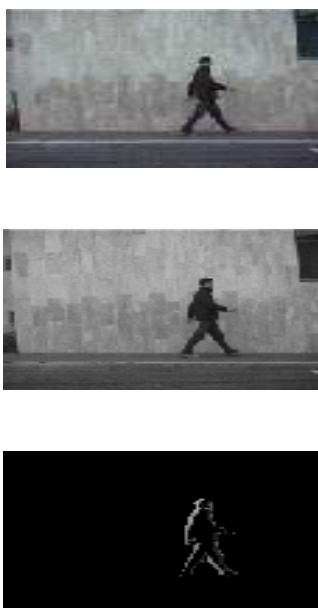
Fig. 1 Object detected using frame difference.
