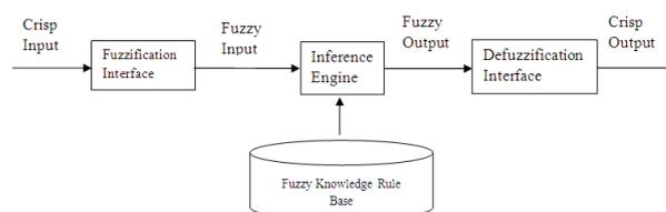
Figure 1: Basic Components of a Fuzzy Expert System
