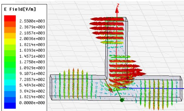
Fig 3: Electric field vector variation when signal entering at port 1
