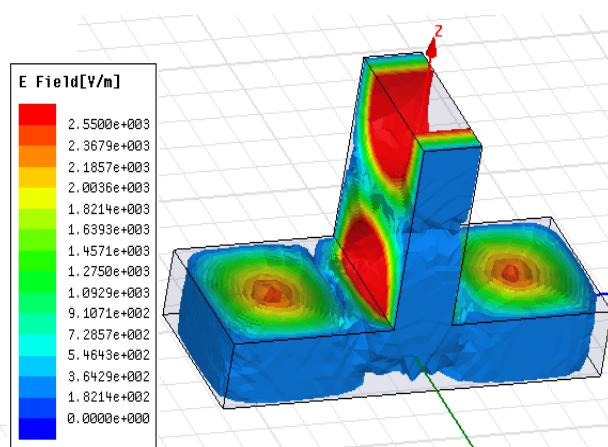
Fig4: Magnitude of field variation when signal entering at port 1
