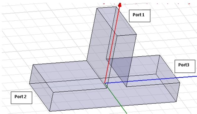
Fig 2: Schematic picture of E plane tee in simulation software
