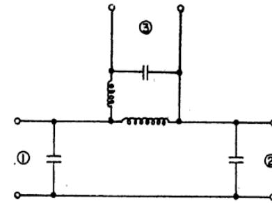
Fig: 1(b) Equivalent circuit of E plane Tee
