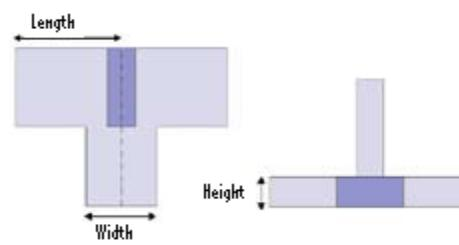
Fig:1(c) Constructional details of E plane Tee
