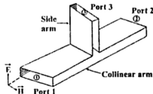
Fig: 1(a) Schematic diagram of E plane Tee
