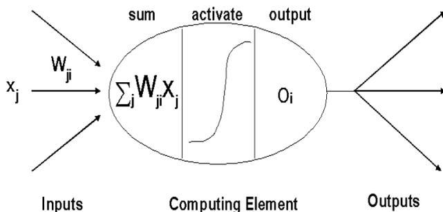
Fig. 2 Back-propagation computing element structure
