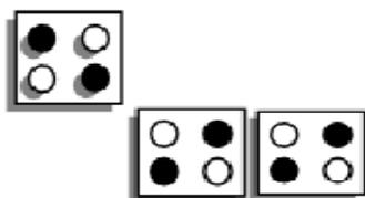
Figure 3. (b) High polarized QCA inverter according to [12]
