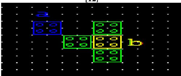
Figure 3. (c) Fault free inverter according to [12]
