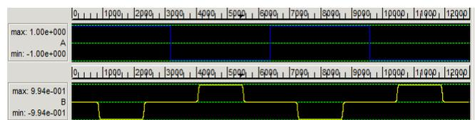
Figure 7. (b) Simulated output of the inverter shown in Fig. 7(a)
