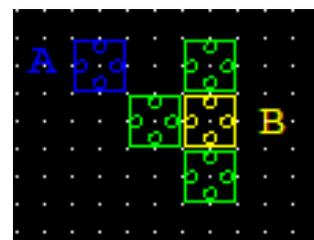
Figure 8. (a) Less faulty inverter using four rotated cells
