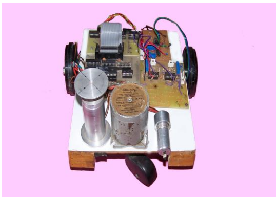
Figure.5: Micro-controller based fiber optic mobile platform
