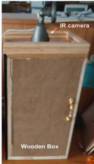
Fig.4. IR camera along with enclosed wooden box.
