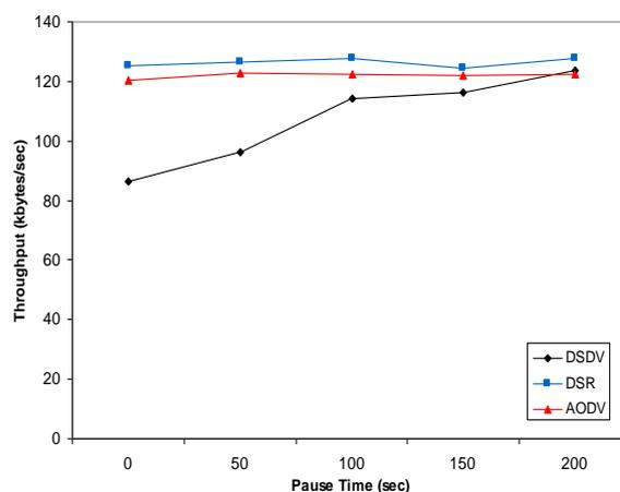
Fig. 2. Throughput vs. node mobility rate (pause time)
