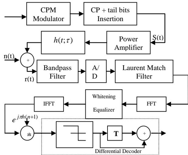
Figure 2. The use of FDE for CPM block diagram with  $h = 1/2$ .
