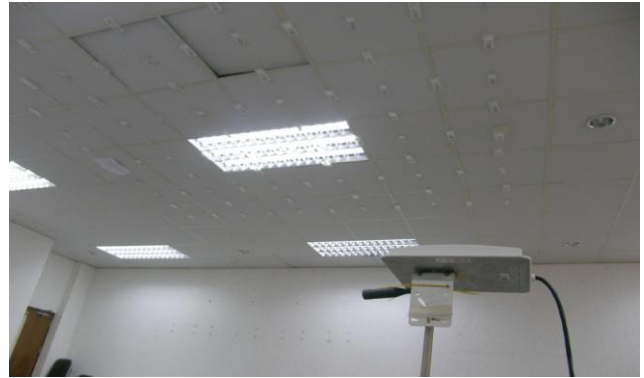
Fig. 3. Reader faces directly up to tags set on the ceiling and used as references and @ngerprints for indoor environment.
