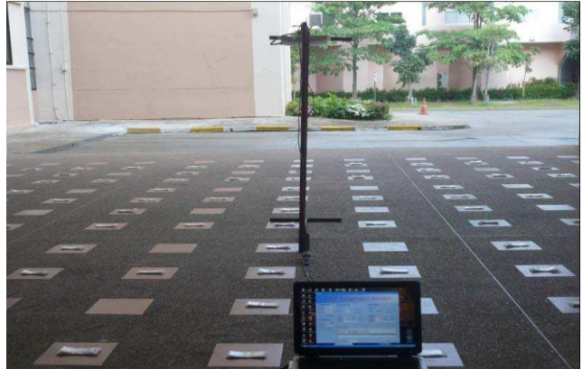
Fig. 4. Reader faces directly down to tags set on the floor and used as references and @ngerprints for outdoor environment.
