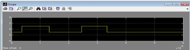
Figure (39) Received 8QAM signal after the decision circuit for Q-Channel
