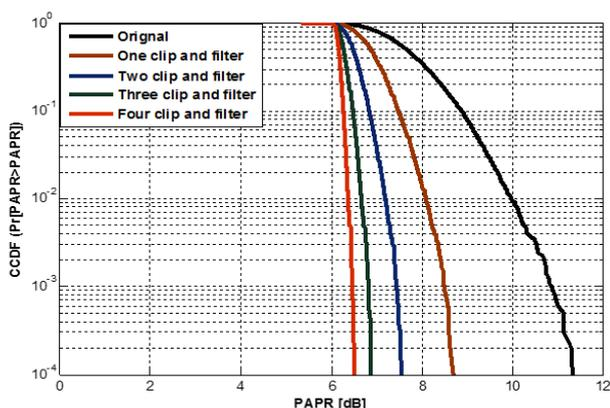
Figure 4. Comparisons of CCDF based on different iteration Clip and Filter techniques
