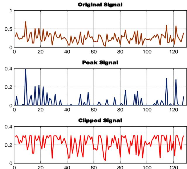
Figure 3. Explain the Original, Peak and Clipped Signal, using Clip and Filter technique
