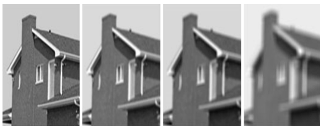
Figure 1. The Produced Scale Space by Gaussian Filter
