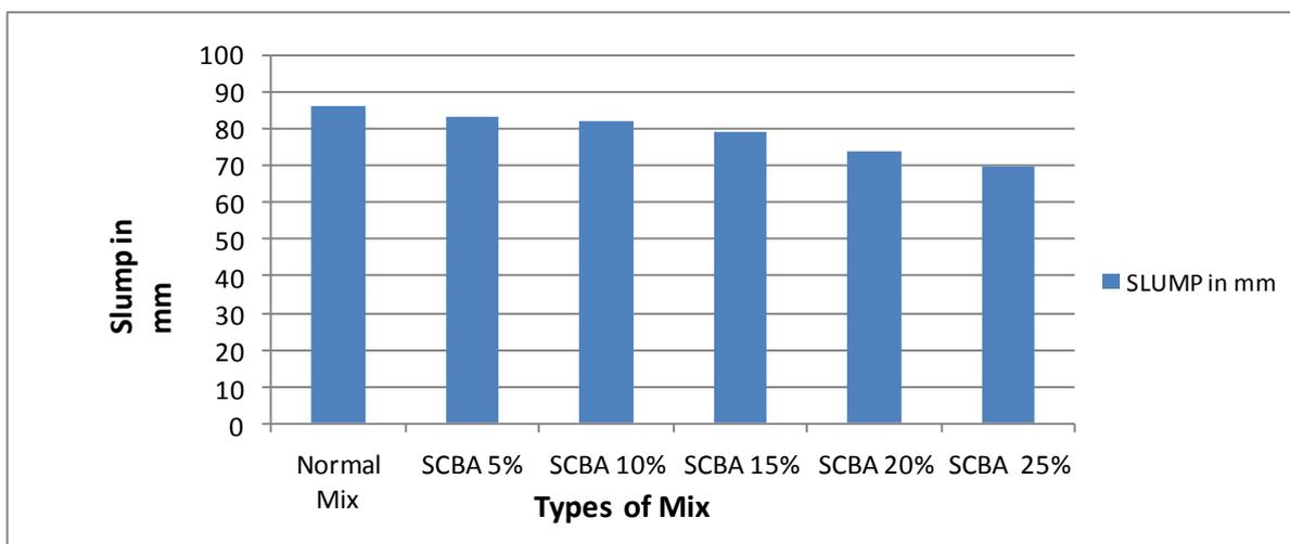
**Slump test vs Mix**
