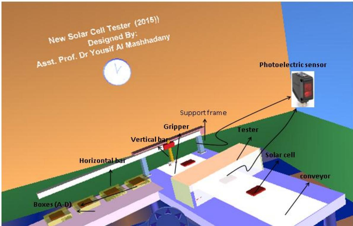
Fig. 1. Design Virtual Reality model for solar cell tester
