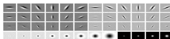
**Fig. 6 An illustration of the LM filter bank that is used to extract texture contrast in the WCE images.**
