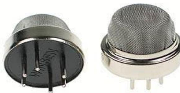
Fig 5: Methane gas sensor
