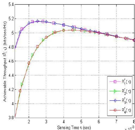
**Figure 4.2: Performance toward sensing time for different necessary interface conditions and channel noise.**
