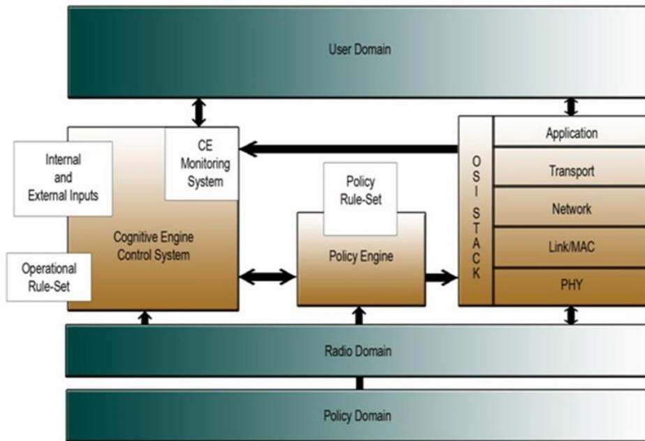
Figure 1: Cognitive Radio Concept Architecture. (Devillers, B., et al2018)
