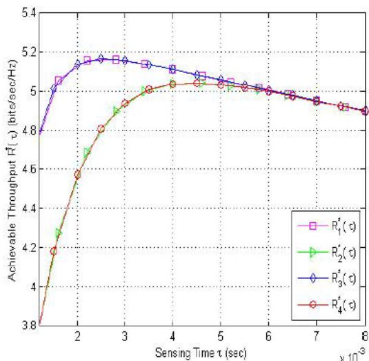
**Figure 4.2: Performance toward sensing time for different necessary interface conditions and channel noise.**
