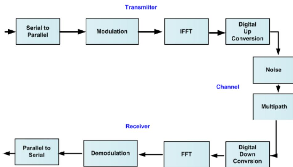
**Figure 2: Orthogonal Frequency Division Multiplexing (OFDM) Architecture. (Hubert, A. et al., 2015)**
