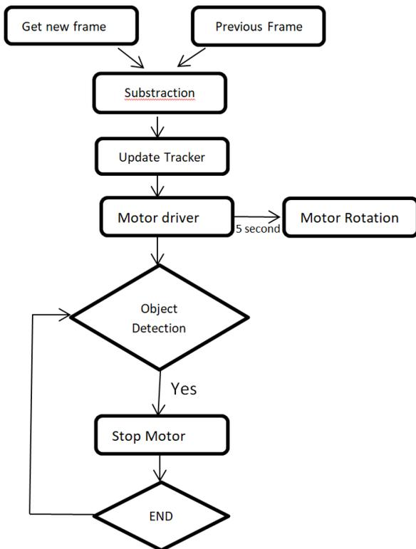
**Figure 2: Flowchart of process**
