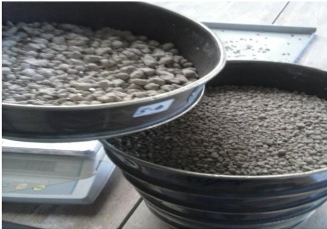
Fig 1. Sieve analysis for Aggregates Source (author 2013)
