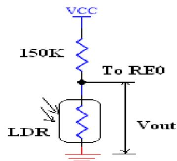
The Light follower makes use of Light Dependent Resistor(LDR). For example, the user can keep two LDR circuits for detecting light coming from front, right and left sides. LDR has a property of varying its resistance according to the intensity of the light falling on it. So if we connect the LDR circuit as shown in Figure to the power supply, the output voltage (Vout) of the circuit will vary according to the amount of light falling on the LDR.[9]
