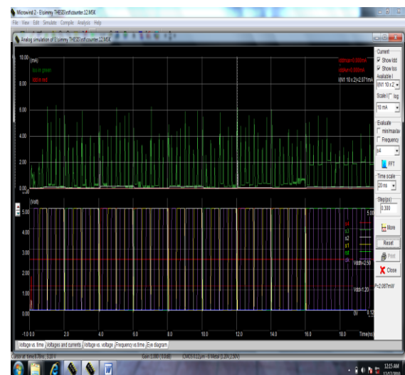
Fig. 10-voltage vs. current waveform of Counter with reset using .12μm technology
