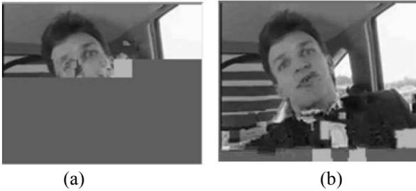
**Fig 8: Comparison of subjective reconstructed video quality for Carphone video sequence at SNR=20.0dB, 64kbps; (a) UEP scheme in [12] ; (b) Proposed UEP scheme.**
