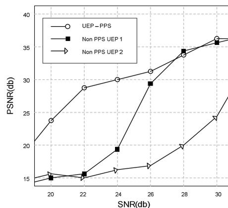
Fig 7: Video Quality in 64kbps; Non-PPS-UEP-1 scheme from [12]; Non-PPS-UEP-2 scheme from [13]
