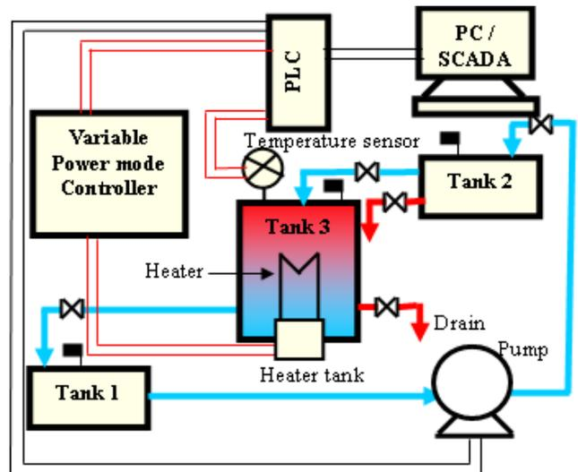
Fig 1.0 Block Diagram of Pilot Plant Experimental setup
