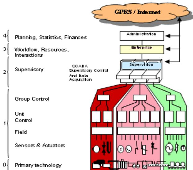
**Fig 2.0 Integrated web based automation architecture**
