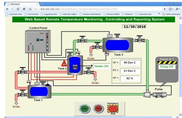
**Fig 8.0 SCADA screen for experimental setup viewed through Internet**
