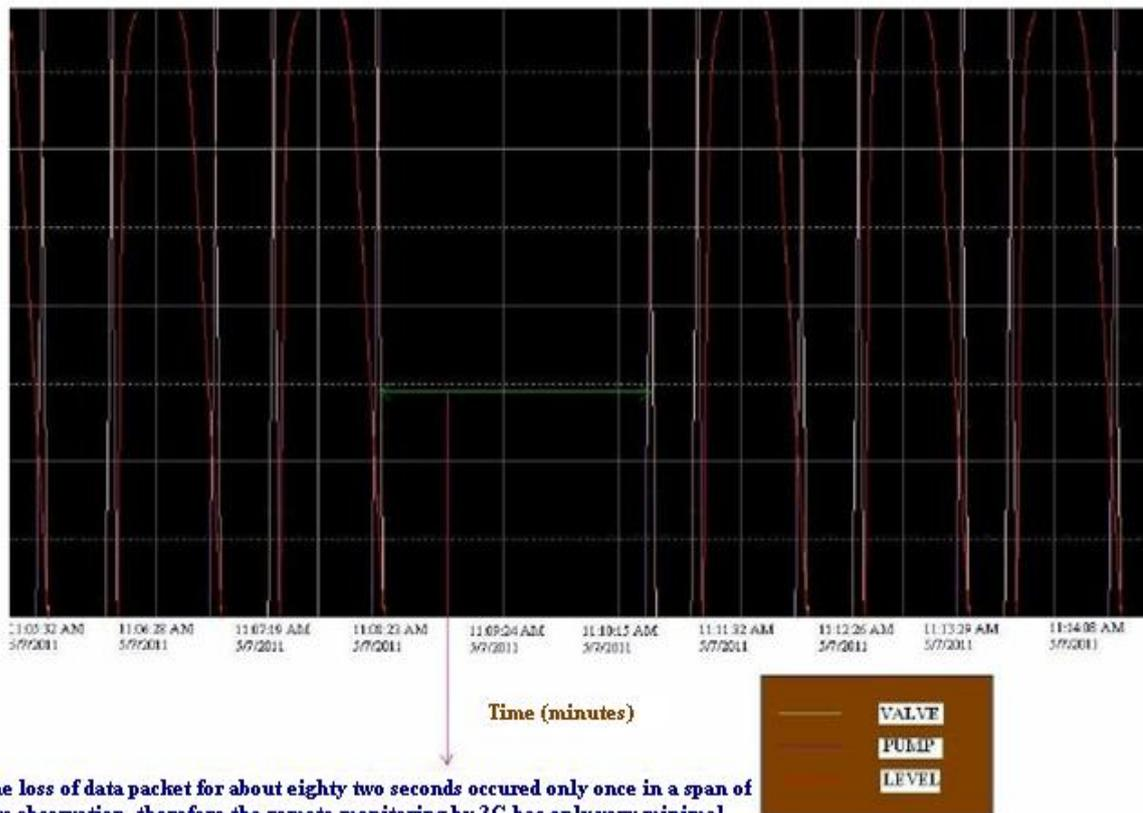
Fig 6.0 Process trend of Pilot plant operation viewed through web browser in 3G environment
