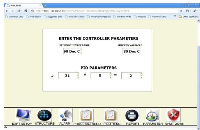
**Fig 9.0 SCADA screen for controller tuning viewed through Internet**
