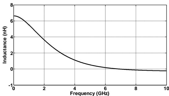
Fig. 5. Simulated inductance of the active inductor
