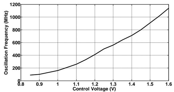
Fig. 6. Oscillation frequency versus control voltage
