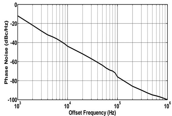
Fig. 7. Oscillator phase noise in 100 MHz oscillation frequency
