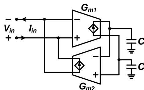
**Fig. 1. Floating Gyrator- C Active Inductor Structure.**
