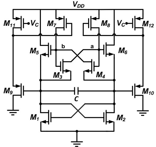
Fig. 3. LC oscillator based on the proposed active inductor
