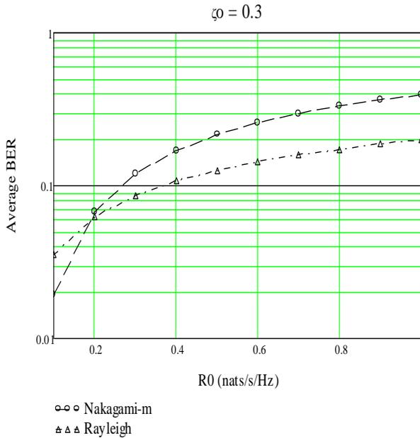
**Fig. 3:** Comparison of upper bound on the average BER of the selected CU versus the target transmission rate  $R_0$  for target outage probability  $\zeta_0=0.3$  of the PU for Nakagami-*m* and Rayleigh fading case.
