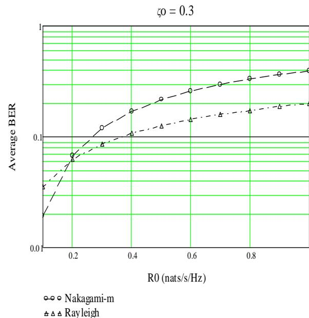
**Fig. 3:** Comparison of upper bound on the average BER of the selected CU versus the target transmission rate  $R_0$  for target outage probabilities  $\zeta_0=0.3$  of the PU for Nakagami- $m$  and Rayleigh fading case.
