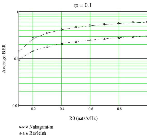
**FIG. 1:** Comparison of upper bound on the average BER of the selected CU versus the target transmission rate  $R_0$  for target outage probabilities  $\zeta_0=0.1$  of the PU for Nakagami- $m$  and Rayleigh fading case.
