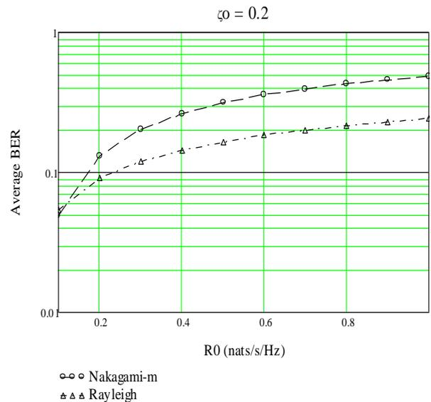
**Fig. 2:** Comparison of upper bound on the average BER of the selected CU versus the target transmission rate  $R_0$  for target outage probabilities  $\zeta_0=0.2$  of the PU for Nakagami- $m$  and Rayleigh fading case.
