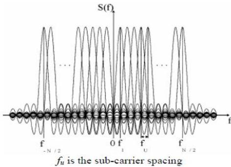
Figure 2: OFDM sub carriers in the frequency domain
