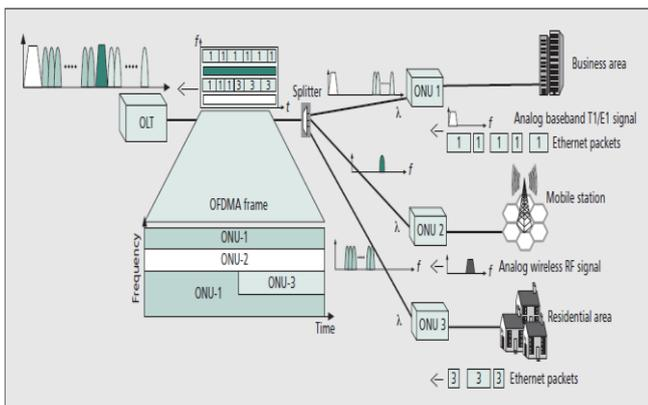
Figure 5: OFDMA PON architecture for delivery of heterogeneous services.
