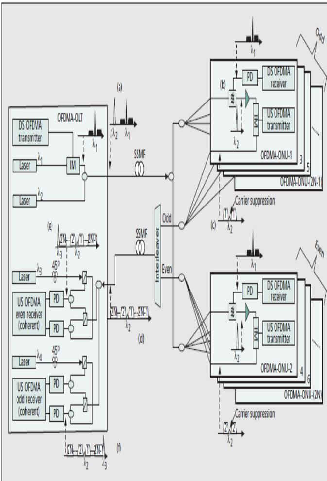
**Figure 7: Upstream OFDMA-PON architecture with source-free ONUs and coherent OLT-side detection.**
