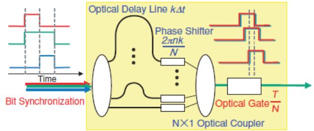
Figure 3: Optical Circuit for Discrete Fourier Transform
