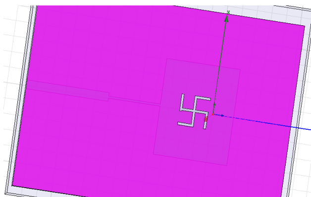
Fig(3.4) View of DGS with Rectangular Patch Antenna for 2.45 GHz
