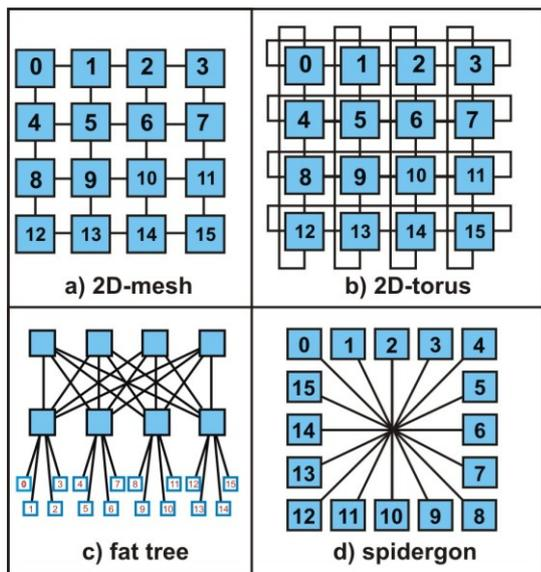
Fig 1: Regular topology based Network-on-Chip
