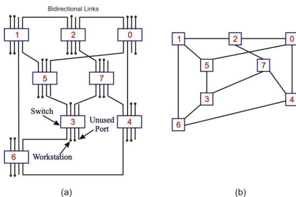
Fig 2: An example application specific NoC with irregular topology having asymmetric structure (a) irregular NoC (b) corresponding topology graph
