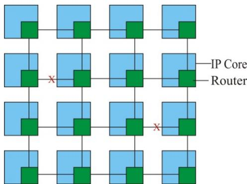
Fig 4: Irregular mesh NoC due to Faults
