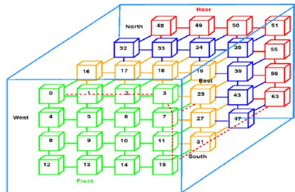
Fig 5: 4x4x4 3D-Mesh based NoC
