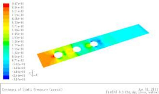
Fig .6. Static pressure of base fin geometry
