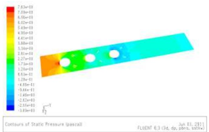
Fig. 8 Static pressure of triangle fin geometry
