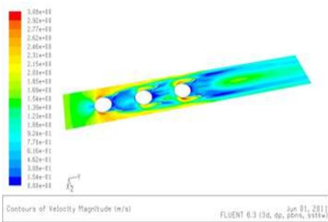
Fig. 5 Velocity magnitude of triangle 45 0
