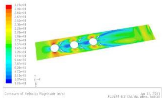
Fig.4 Velocity magnitude of rectangle 45 0
