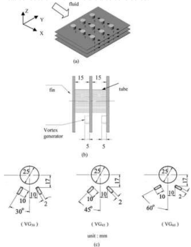
Fig.1. Physical model and relevant geometrical dimensions of the vortex generators. (a) Physical model (top view), (b) side view, and (c) three different span angles.
