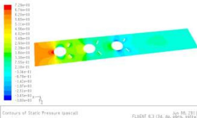
Fig. 7 Static pressure of rectangle fin geometry
