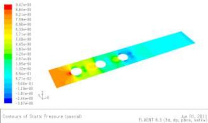
Fig .6. Static pressure of base fin geometry
