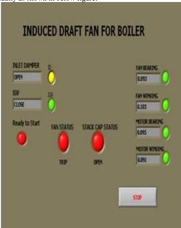
Fig-7 Inlet Damper Open Condition
