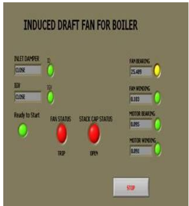
Fig-9 Fan Bearing Temperature. Beyond limit
