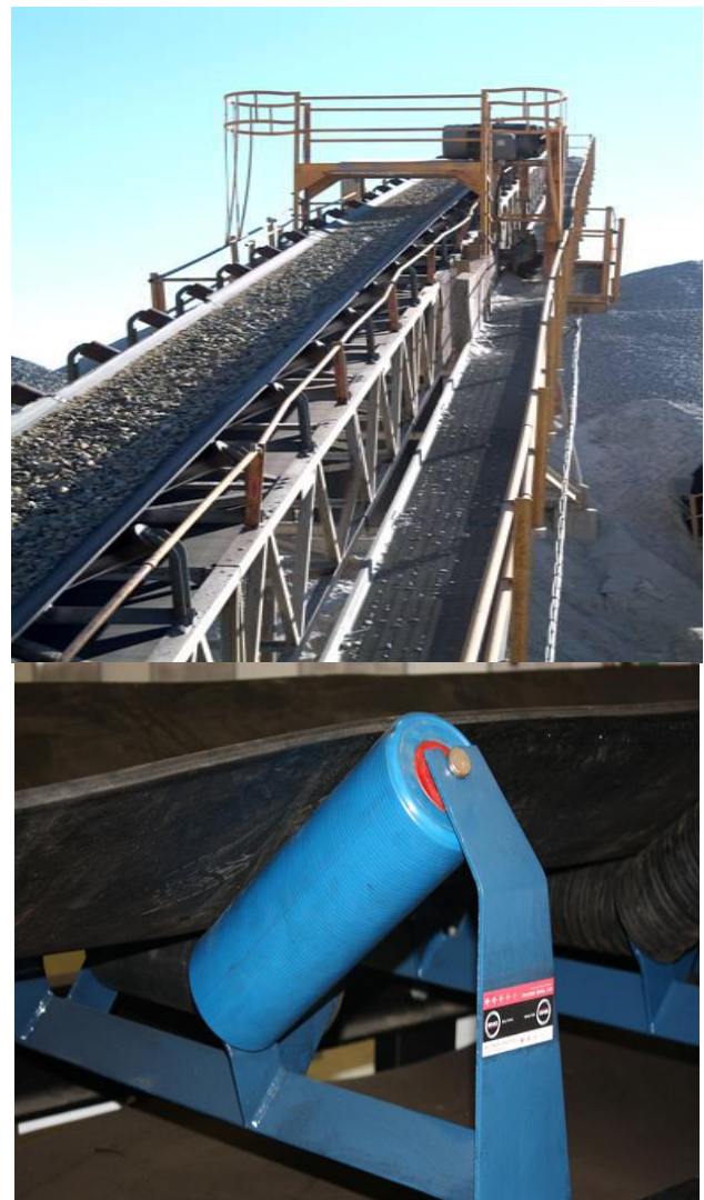
Figure 1: Typical idler roller used in conveyor system in mining and similar industries
