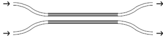
Fig 1.3 Directional Coupler Switch
