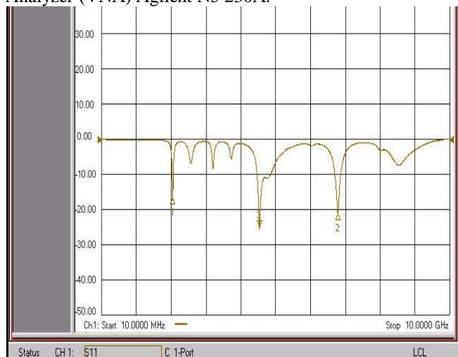
Figure 11: Measured return loss for proposed antenna.
