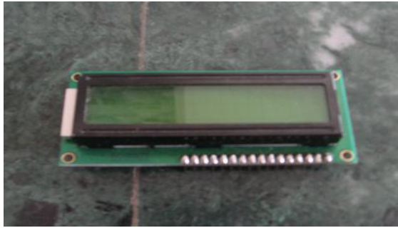
Fig 6: This is Simple 16*2 LCD which is used for displaying alphabets.
