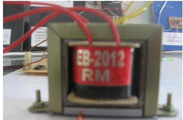
Fig 4: This is Step down Transformer which actually steps down the voltage level.
