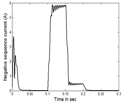
**Fig. 16 detecting negative sequence current with model two**
