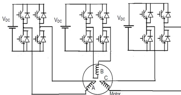
Fig. 2 Feeding PMSM from separate phases
