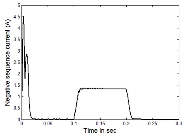
**Fig. 5 detecting negative sequence current with model one**
