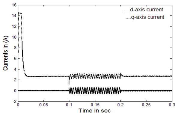
**Fig. 8 Idq -axis current with model two**
