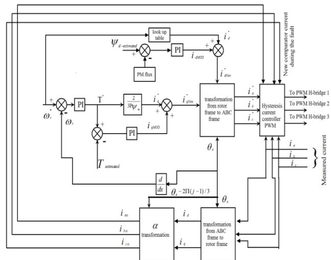
**Fig.4. Remedial operation of PMSM at fault (second model)**
