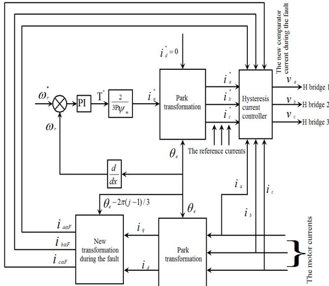
**Fig.3. Remedial operation of PMSM at fault (first model)**
