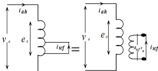
Fig.1 Represented the turn to turn fault
