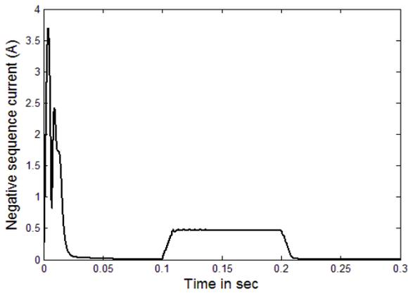
**Fig. 6 detecting negative sequence current with model two**
