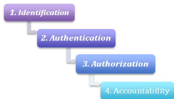
Fig. 1 Primary elements of access control
