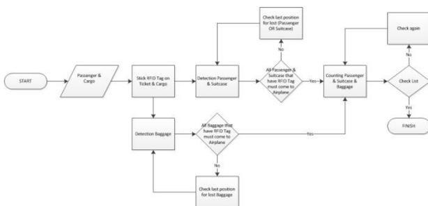
**Fig. 1 System Overview for one way flight.**
