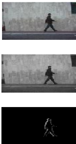
Fig. 1 Object detected using frame difference.
