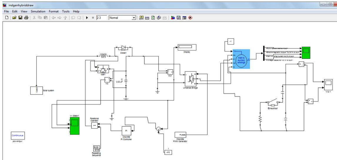
Figure 9. Hybrid solar/wind scheme with fuzzy controller in simulink (version 7.9.0.529)
