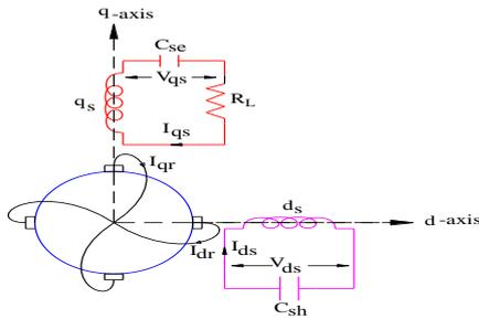
Figure 3: Circuit representation of the single-phase in d-q axes stationary reference frame
