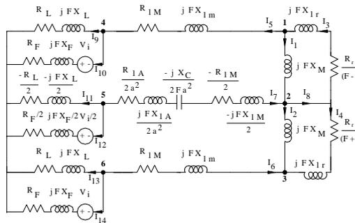
Figure 4: Equivalent circuit of SESPIG
