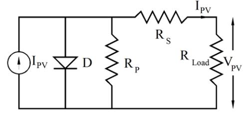
Figure 2: Equivalent circuit of PV cell
