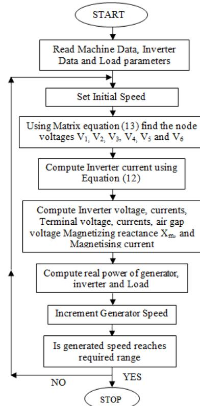
Figure 8. Flowchart for steady-state response
