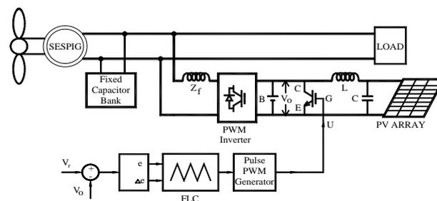
Figure 1. Schematic diagram of solar-wind hybrid scheme
