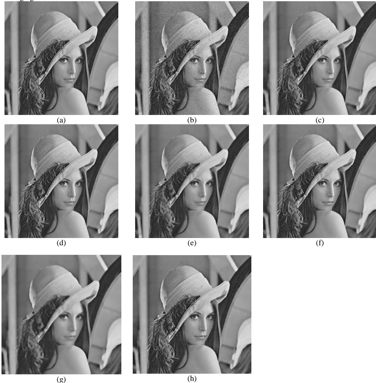
Figure 4 (a) Original Image (b) Noisy Image (c) 3x3 Median Filter (d) 3x3 IQR Filter (e) 5x5 Median Filter (f) 5x5 IQR Filter (g) 7x7 Median Filter (h) 7x7 IQR Filter
