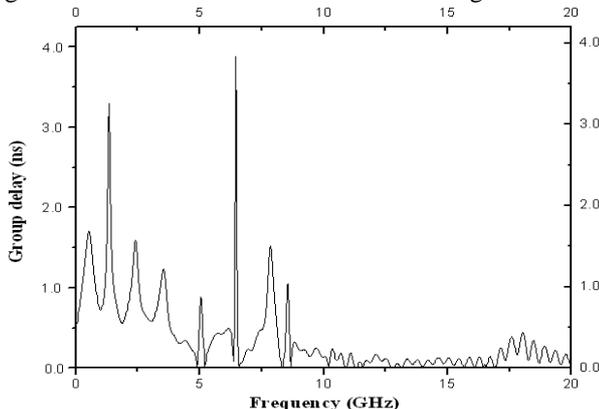
Fig. 9 Variation of group delay vs. frequency of SPQSMA
