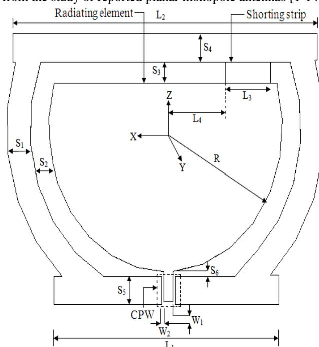
Fig. 1 Geometry of SPQSMA:  $L_1=96$  mm,  $L_2=130$  mm,  $L_3=25$  mm,  $L_4=20$  mm,  $W_1=4$  mm,  $W_2=1$  mm,  $S_1=10$  mm,  $S_2=8$  mm,  $S_3=8$  mm,  $S_4=10$  mm,  $S_5=10$  mm,  $S_6=1.5$  mm,  $R=50$  mm
