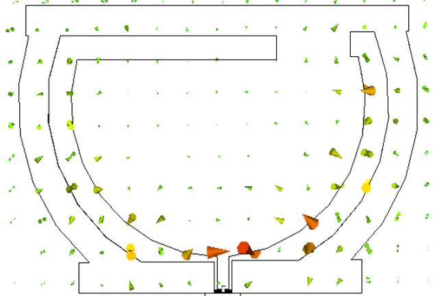
Fig. 11 H field distribution of the antenna
