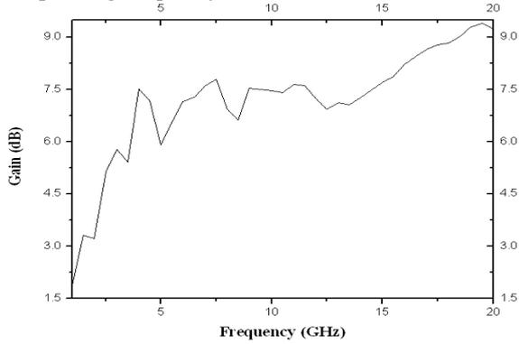
Fig. 7 Variation of maximum gain vs. frequency of SPQSMA
