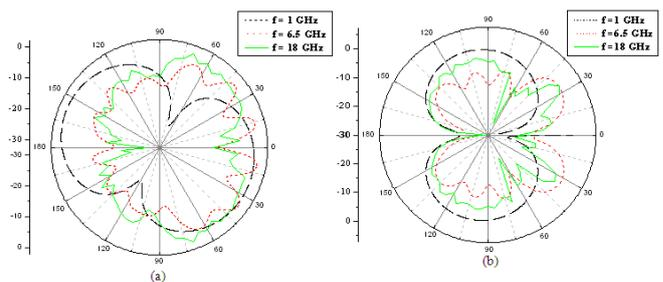
Fig. 5 Farfield radiation pattern at frequencies 1GHz, 6.5 GHz and 18 GHz for (a)  $\Phi = 0^\circ$  and (b)  $\Phi = 90^\circ$
