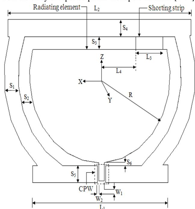
Fig. 1 Geometry of SPQSMA:  $L_1=96$  mm,  $L_2=130$  mm,  $L_3=25$  mm,  $L_4=20$  mm,  $W_1=4$  mm,  $W_2=1$  mm,  $S_1=10$  mm,  $S_2=8$  mm,  $S_3=8$  mm,  $S_4=10$  mm,  $S_5=10$  mm,  $S_6=1.5$  mm,  $R=50$  mm
