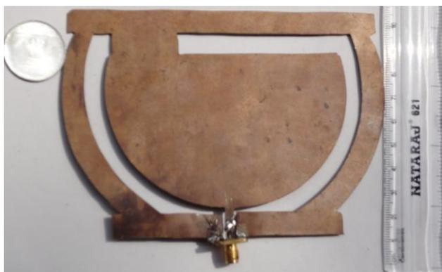
Fig. 14 Photograph of the fabricated SPQSMA
