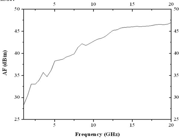
Fig. 8 Variation of AF vs. frequency of SPQSMA
