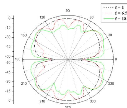
Fig. 6 Far field radiation pattern at frequencies 1 GHz, 6.5 GHz and 18 GHz for  $\theta = 90^\circ$
