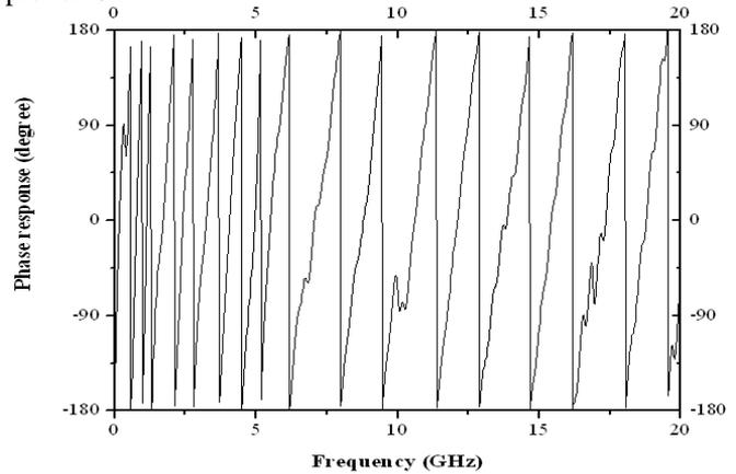
Fig. 10 Variation of phase response vs. frequency of SPQSMA
