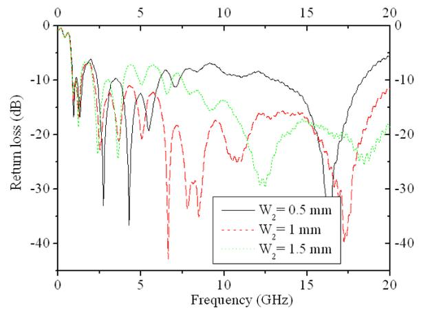
Fig. 4 Return loss characteristic of the antenna for different values of  $W_2$
