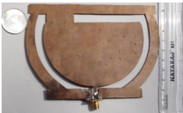
Fig. 14 Photograph of the fabricated SPQSMA
