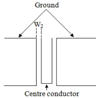
Fig. 3 Design of the proposed CPW line
