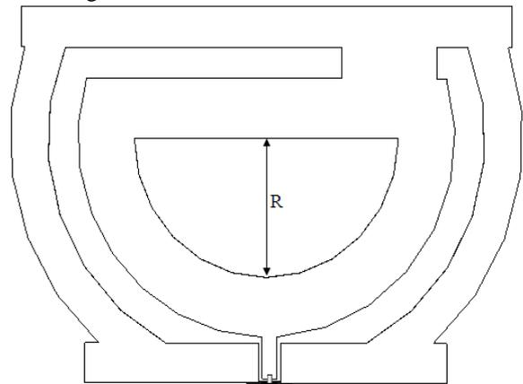
Fig. 12 Geometry of the proposed antenna with slot
