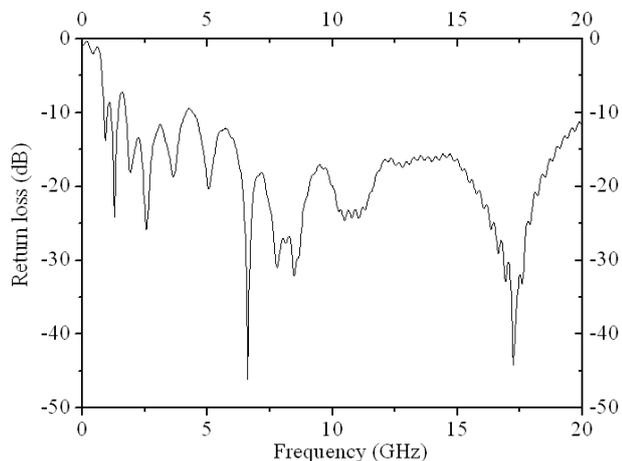
Fig. 13 Return loss characteristic of the proposed antenna with slot
