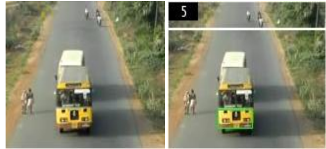
Fig 7: Failed case to detect due to occlusion
